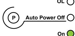
While the external power supply is present, automatic power off is disabled. But if the supply is cut off, the batteries take over and automatic power off acts at the end of 10 minutes.
