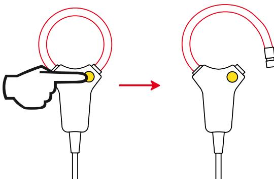
Open it and place it around the conductor carrying the current to be measured (only one conductor in the sensor). Close the coil. You must hear the "click".
