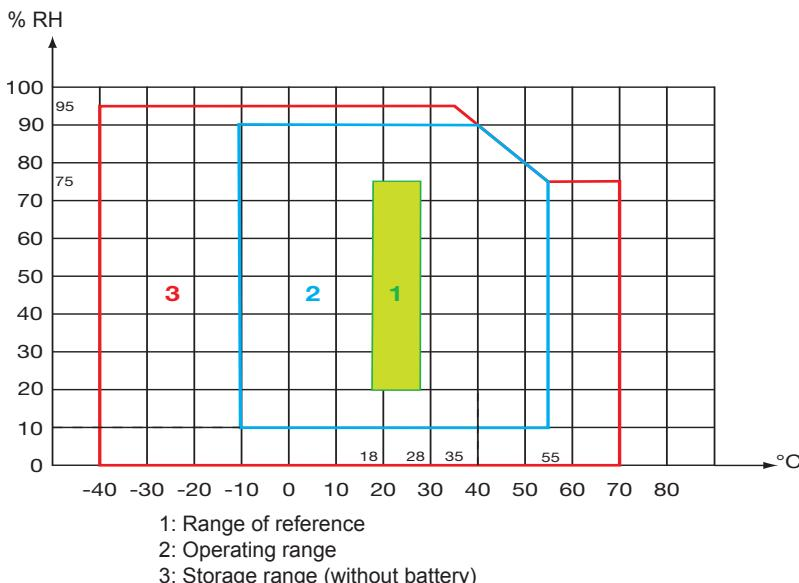
For an extended period of non-use or storage, withdraw the batteries from the electronic unit. The sensor by itself can withstand a maximum temperature of 90°C for 10 minutes.
