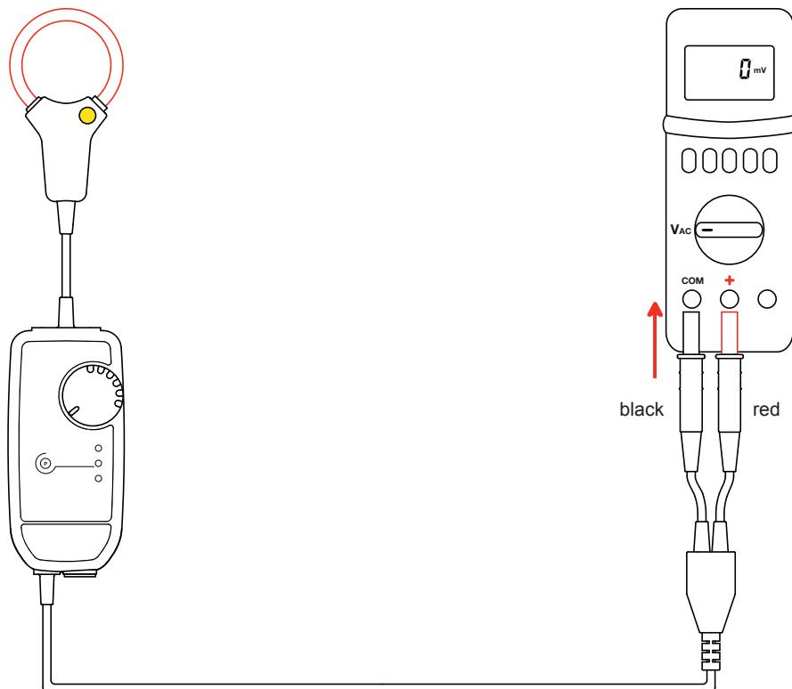
Put the electronic unit into operation by turning the switch to some position. The green **On** indicator starts blinking.
