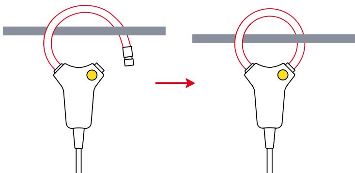
To optimize measurement quality, centre the conductor in the coil.
