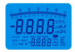
The large double LCD display with blue backlighting also offers a 61+2-segment full-scale bargraph. The Central Zero function allows you to view variations immediately. This type of bargraph is particularly practical for making adjustments.
