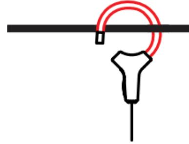
In order to optimize measurement quality, it is best to centre the conductor in the coil and to make the shape of the coil as nearly circular as possible.
