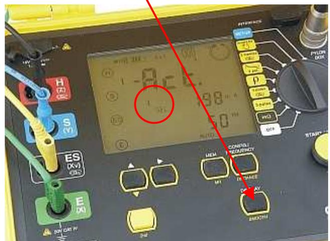
Check the current in each pylon leg by switching to channel 1,2,3 and 4 - in this way you can find corroded (or not connected) earth connections (no current is flowing).
