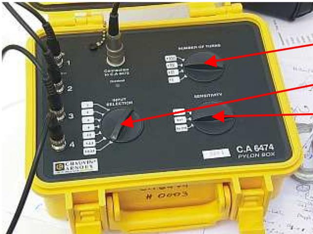
Check the rotary switches on CA6474:
