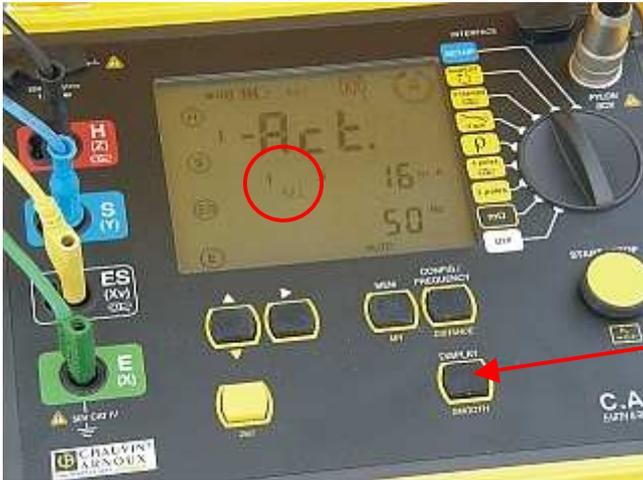
Switch with DISPLAY-key to  $I_{SEL}$ , which is the total pylon earth current, measured by the 4 Rogowski coils (channels 1+2+3+4 selected)
