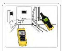
**Detection of metal water pipes**
