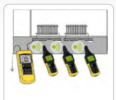
**Detection of metal heating ducts**
