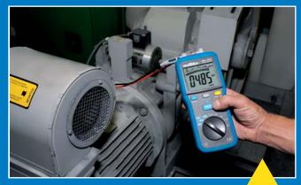
Measuring insulation on a motor for preventive maintenance
