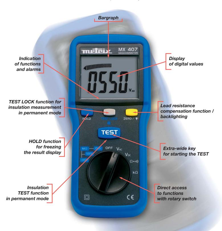
**Safety** The MX 407 is a safe instrument. If a dangerous voltage is present, it is detected automatically. Insulation measurements for voltages greater than 25 V are automatically inhibited, making measurement impossible if there is any danger.
