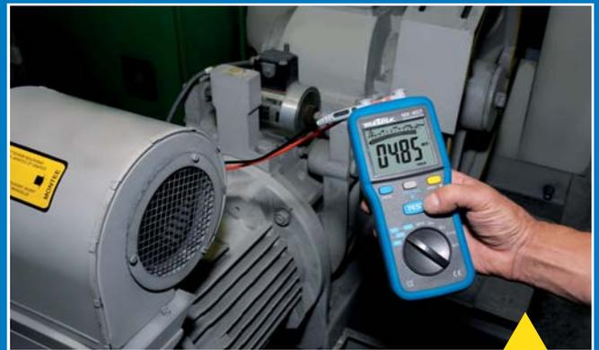
Measuring insulation on a motor for preventive maintenance
