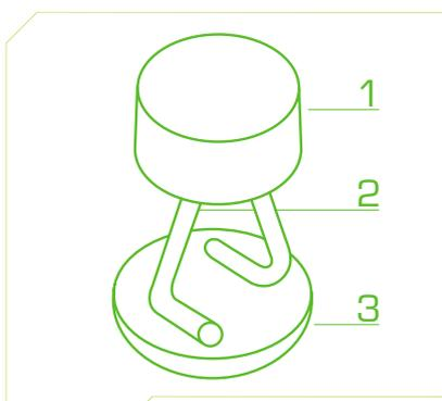
The end of the sensor's body (1), the thermocouple fins (2) are brazed onto a tip (3).
