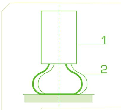
At the end of the sensor's body (1), the thermocouple fins (2) are soldered and guarantee proper application of the hot point to the surface. Some models marketed with the "surface sensors" description give errors that can be more than 20 °C at high temperature (300 °C). Below is an example of a contact-type surface temperature sensor that is not suitable for measurement purposes\*\*:
