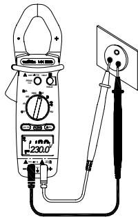
Connect the red test lead to the "+" input terminal and the black test lead to the "COM" input terminal.
