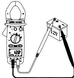
Press on the  $\sim/\equiv$  button to display the  $\equiv$  symbol (direct signal).
