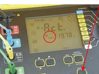
Switch with DISPLAY-key to  $I_{\text{SEL}}$ , which is the total pylon earth current, measured by the 4 Rogowski coils (channels 1+2+3+4 selected)
