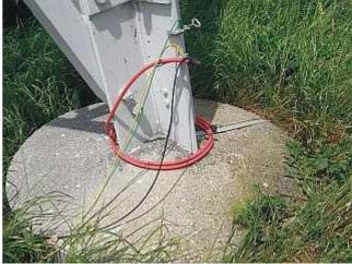
Connect Current (E) and voltage (ES) sockets with the tested Earth system using separate cables, connection points should lay side by side and above the Rogowski (Ampflex) coil.
