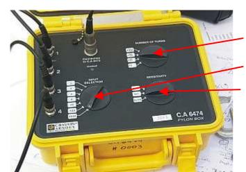
Check the rotary switches on CA6474:
