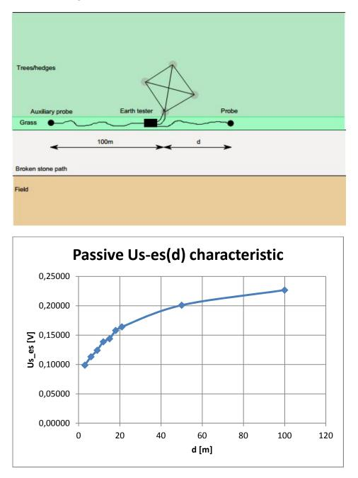
Uh-e remained quite constant when relocating the probe, Us-es rose with distance from pylon (Obj. 1/Tst. 2+5-12). This could mean that there was less ground resistance north of the pylon (maybe due to buried tubes or cables?) and that the **potential funnel of the pylon for the 50Hz noise currents reached even beyond 100m south of the pylon**. The low Us-es value in Obj01/Tst13 was probably a measurement error (compare with Obj01/Tst21+22)...
