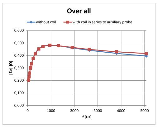
⇒ Therefore one must take care to always fully uncoil the cable coil for the auxiliary probe connection!
