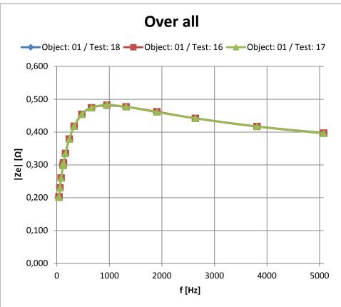
The selective measurements into pylon top and ground are all reproducible and show smooth curves, speaking of the quality of the measurement. The curves into the top earth rope are almost linear, showing very nice the inductance of the earth rope. **Local earth resistance is approximately 0.4 Ohms**, which is quite good.
