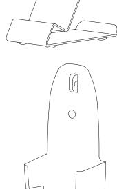
It is attached to the wall. It can be used to protect the device against theft by adding a padlock.
