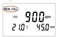
Any recording in progress is then stopped, and it is impossible to restart recording before emptying the memory.
