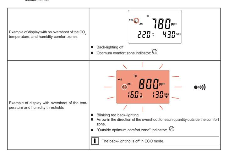
For the **1D** and **3D** modes, if the buzzer is active, it will sound intermittently upon the appearance of the  $\stackrel{\bigodot}{\bigcirc}$  symbol.
