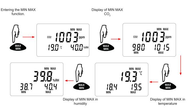
When the MIN MAX function is activated, recording of the minimum and of the maximum starts but the display of the three quantities measured makes it possible to continue using the device normally.
