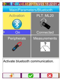
To use this function, you must first activate it from the Main/Parameters/Bluetooth menu by setting the Activation to "On" (validate the item with F2 У, to allow item
