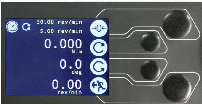
◀ Clear colour display of status, clockwise and anticlockwise speeds, position and torque.
