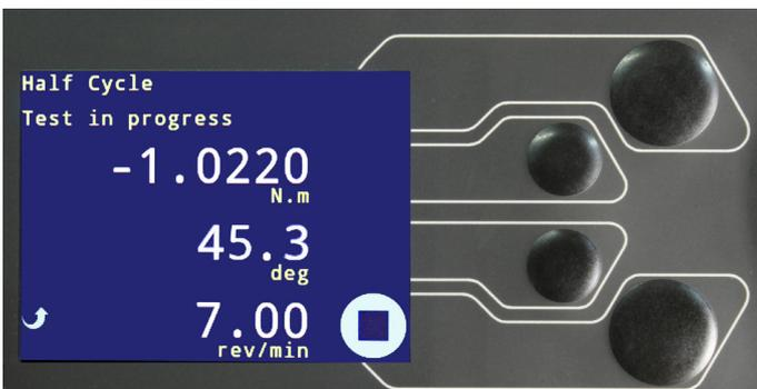
◀ Continuous live readings during testing, including status and cycle count, plus peak and break capture by AFTI, or full data capture and plotting with VectorPro™ Lite.
