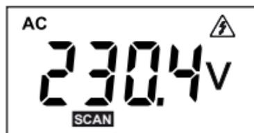
If the voltage is  $> 30V$ , the instrument displays
