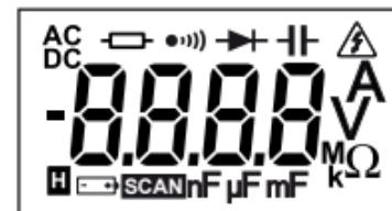
If the battery voltage is too low for correct operation of the instrument, the  $\ominus +$  symbol is displayed.
