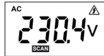
If the voltage is > 30V, the instrument displays indicating that the voltage is dangerous.
