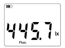
The sensor has no memory effect and is not dazzled, so you can make a low-illumination measurement just after a very-high-illumination measurement.
