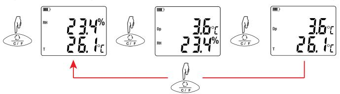
The last display selected is saved when the instrument is switched off.
