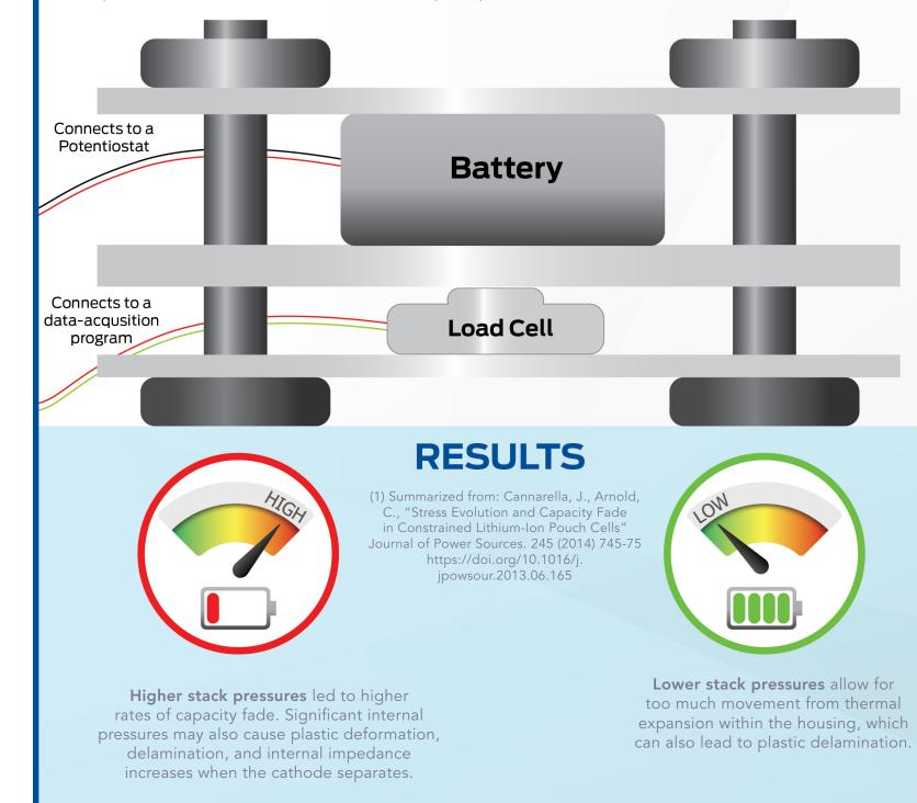
Pressure mapping has been used in multimonth studies evaluating the pressure profile during thousands of charging and discharging cycles — principles that can be applied to evaluating battery housing materials.
