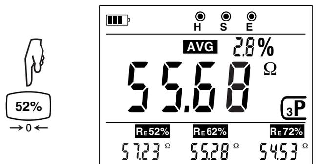
The instrument immediately calculates the mean of the 3 measurements and the percent difference between the lowest value and the highest value. For the measurement to be valid, the difference must not exceed 5%.
