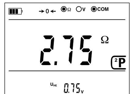
The  $\rightarrow 0 \leftarrow$  symbol blinks during the compensation. When it is done, the display unit indicates **00.00 $\Omega$** .
