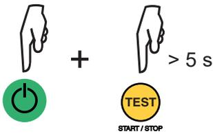
To do this, keep the **On/Off** and **TEST** buttons pressed for more than 5 seconds when switching on; the names of the H, S, E terminals become C, P, X. This information is preserved even if the instrument is switched off.
