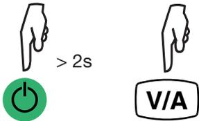
Long-press the **On/Off** button to switch the instrument on.
