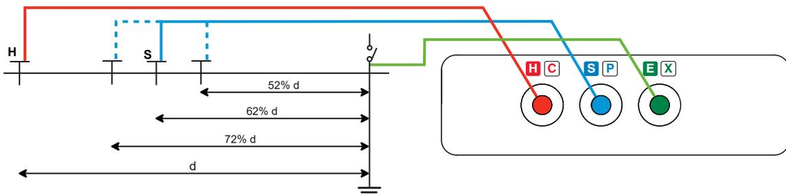
The 3 measurement results must be the same to within a few percent. If this is the case, the measurement is valid. If not, it is because the S rod is in the zone of influence of the earth electrode.
