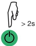
Long-press the **On/Off** button to switch the instrument on. It indicates that it is in resistance measurement mode by displaying **2P**.
