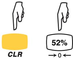
Pressing the  $\rightarrow 0 \leftarrow$  key deactivates or reactivates the compensation of the leads.
