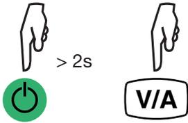
Long-press the **On/Off** button to switch the instrument on.
