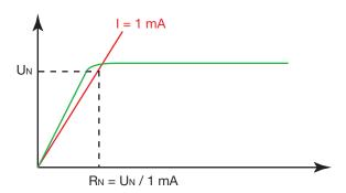
The voltage developed as a function of the resistance measured has the following form: The maximum load capacitance is 300nF, but the instrument operates correctly up to  $2\mu F$ .
