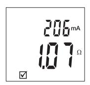
To make sure that there is no voltage, make a voltage measurement before the continuity measurement.
