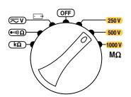
Set the switch to one of the  $M\Omega$  positions.
