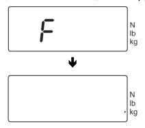
After adjustment the balance turns itself off again automatically.
