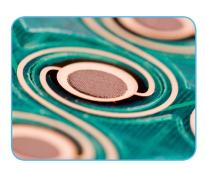
Flexible Sensor Design – As the name suggests, the CONFORMat conforms to the subject and seating interface ensuring consistent and accurate results. The sensor contains over 2,000 sensing elements that can move independently of each other in three dimensions, giving the most accurate interface pressure measurements.
