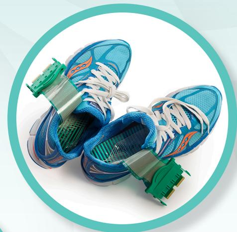
In-shoe pressure measurement systems uses pressure and timing data to reveal what's happening inside the shoe.
