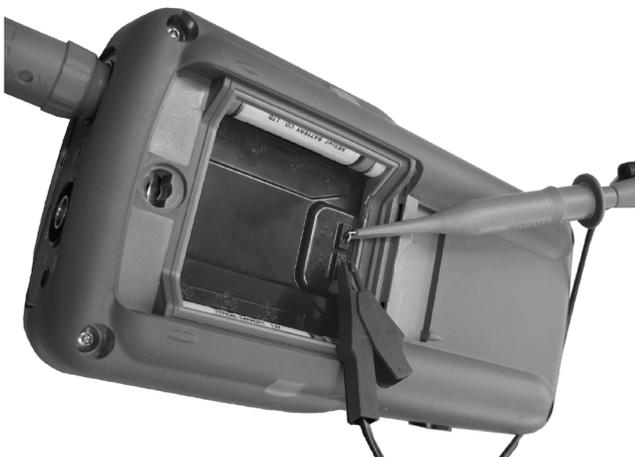
Connect the sensor to be adjusted to the calibration output under the battery housing cover, as shown opposite.
