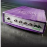
The **E4000** and the **M600** require the X4 InterX Unit as the interface to the computer.
